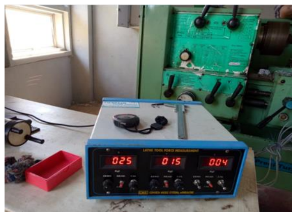
Figure 2 Lathe and Tool Dynamometer to Record Cutting Forces
