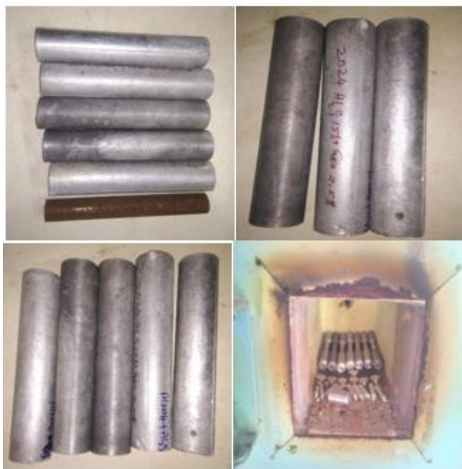
Figure 1 Composite Rods and Heat Treatment of Material for Hardening
